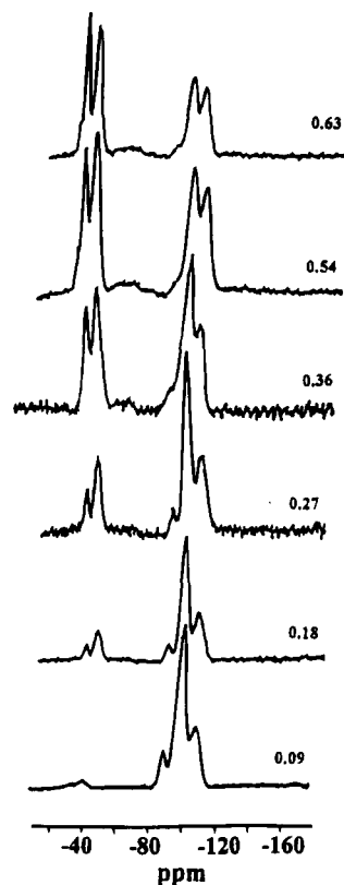
Figure 2. 29 Si NMR spectra of various DPMOS–TMOS gels compositions (numbers indicate molar ratio of DPMOS).
